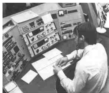
The Ajax's were no frills basic transmitters. Back-up was via a Marconi H1000 which had all the spot frequencies feeding a wide band amplifier into a matched Mast Radiator aerial. The times when on nights, listening to our local ships voyaging in the Med, calling Cagliari/IDC without success and jumping in to work them were now numbered. SSB somehow did not seem to pack the same 'punch' as DSB.
